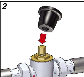
◀ Fitting cap for temperature adjustment
