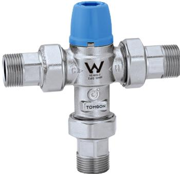
The tempering valve is used to regulate the set temperature of mixed hot and cold water even when variations occur in the water supply conditions.
